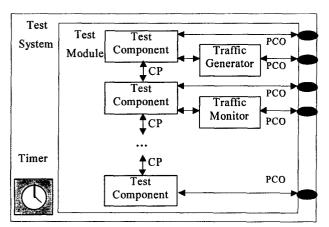
Figure 2.2 Conceptual model of a protocol performance test system
