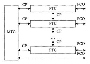
Figure 2.1 Conceptual model of test components
