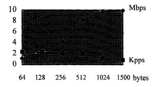
Figure 4.2 Throughput of one port of Cisco 4700
