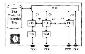
Figure 4.1 Architecture of a protocol performance test system
