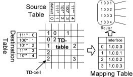
Fig. 5: FIST: A forwarding table structure for TwoD-IP
