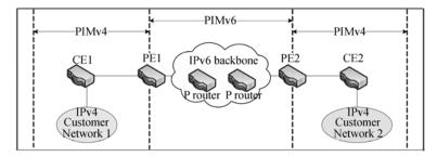
Figure 3 4over6 multicast components.
