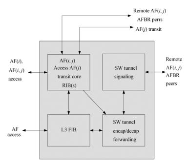
Figure 2 Softwire AFBR reference model.
