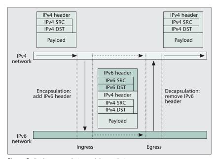
Figure 2. Packet encapsulation and decapsulation.
