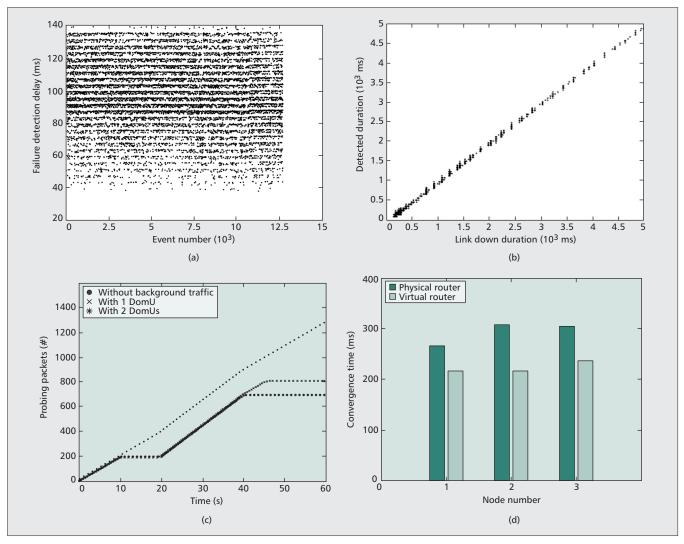
Figure 5. Failure detection performance in testbed: a) (experiment 1) failure detection delay; b) (experiment 2) failure duration; c) (experiment 3) detection overhead; d) (experiment 4) OSPF convergence.
