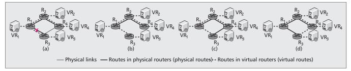
Figure 1. An example: inconsistency between physical and virtual routes occurs at different stages after network failure occurs: a) stage 1: consistency between physical and virtual routes before failure; b) stage 2: inconsistency between physical and virtual routes after failure detection; c) stage 3: inconsistency between physical and virtual routes after rerouting; d) stage 4: inconsistency between physical and virtual routes after failure recovery.
