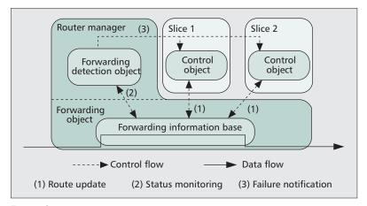
**Figure 3**. *The internal implementation of each VegaNet node.*
